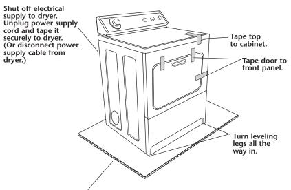
Slide dryer onto cardboard or hardboard before moving it across the floor to prevent damaging floor covering.
